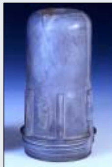
No corrosion with Alocrom treatment.
