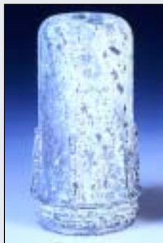
Rapid corrosion of untreated aluminium.
